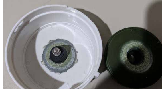
B. Condition of the impeller ruined for ABSENCE OF WATER
