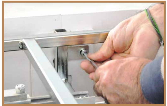
STEP 2: Unscrew the 4 screws using the suitable key to remove the rear wooden cover
