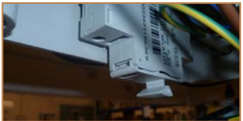
Fig. 2 - Fuse for heating plate (10A or 16A) This fuse is situated in the control box. Unscrew the 4 screws from the control box cover to change this fuse.
